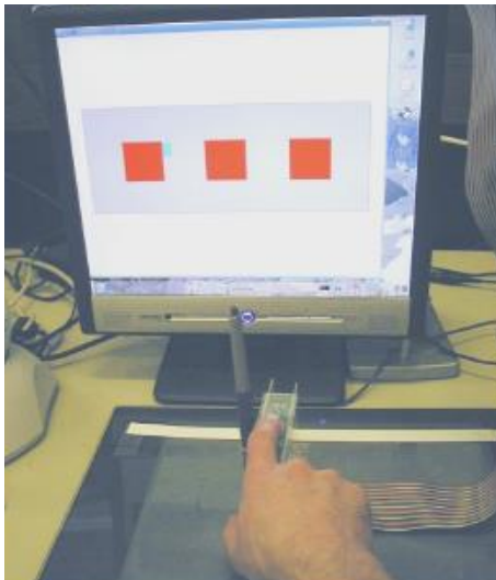
Figure 3. The 2D workspace, showing the index finger resting on the tactile stimulator, the graphics tablet which provides positional information and the visual display which shows the position of the exploring finger in relation to the surfaces available for exploration.
